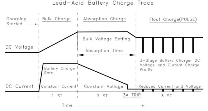
Step 1 : Bulk charge - bring batteries to 75% capacity fast.
