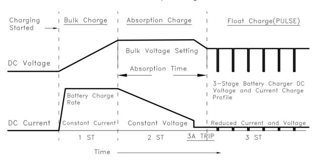
Lead-Acid Battery Charge Trace
