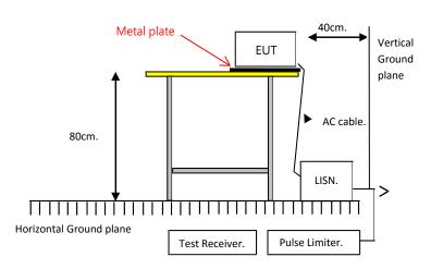
Figure 1: System Deployment of EMI Test
