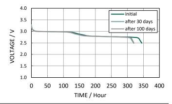
Charging Condition : CV(3.4V, 560 $\Omega$ , 48H, 60°C) Discharging Condition : CR(100k $\Omega$ , 60°C)
