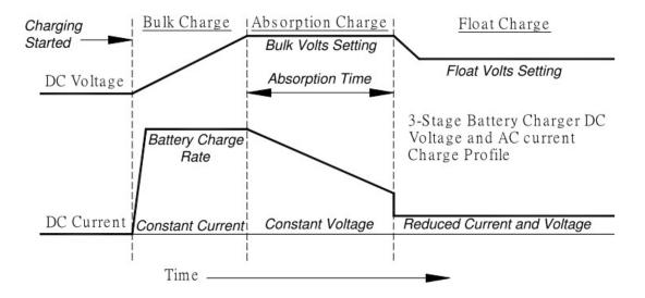
Step 1 : Bulk charge – bring batteries to 75% capacity fast.
