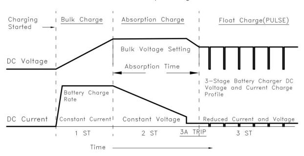
Lead-Acid Battery Charge Trace
