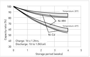
Self-discharge is affected by the temperature at which
